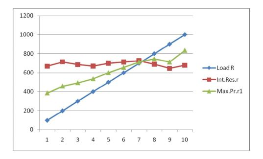
Here the load line R intersects at the two intersecting point of the internal resistance r and maximum power transfer resistance r1 at a value of 713.5 ohms.
