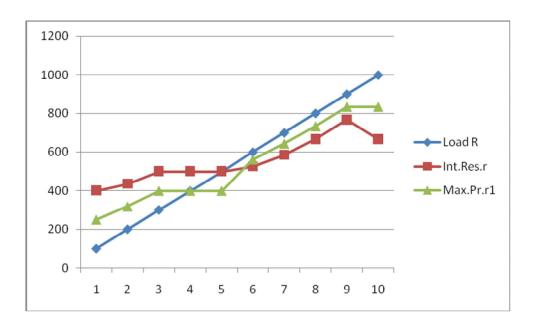
Here the load line R intersects the internal resistance line r at value of 500 ohms quite nearer (possibly due to some experimental errors) to the intersecting point of the two resistance line of internal resistance r and maximum power transfer resistance  $r_1$ .
