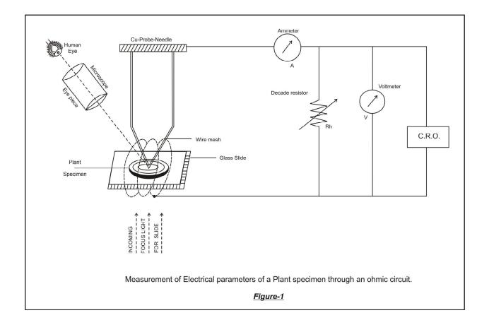
In the Ohmic circuit, a miliammeter for measuring the electrical current I and an external variable load resistor R are attached in series with the sample electrical source of plant's section(under experiment). Further, a D.C. voltmeter along with an Oscilloscope (for more accuracy) is attached across the load resistor R to measure the EPD in volts. Now several transverse sections of its stem cell are obtained by cutting it into the thickness of nearly 0.5 micron.
