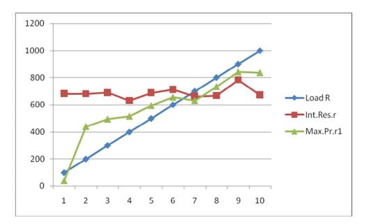
Here the load resistance line R intersects internal resistance line r at the value of 662.5 ohms quite nearer (possibly due to some experimental errors) to the intersecting point of 631.2 ohms of internal resistance r and maximum power transfer resistance  $r_1$
